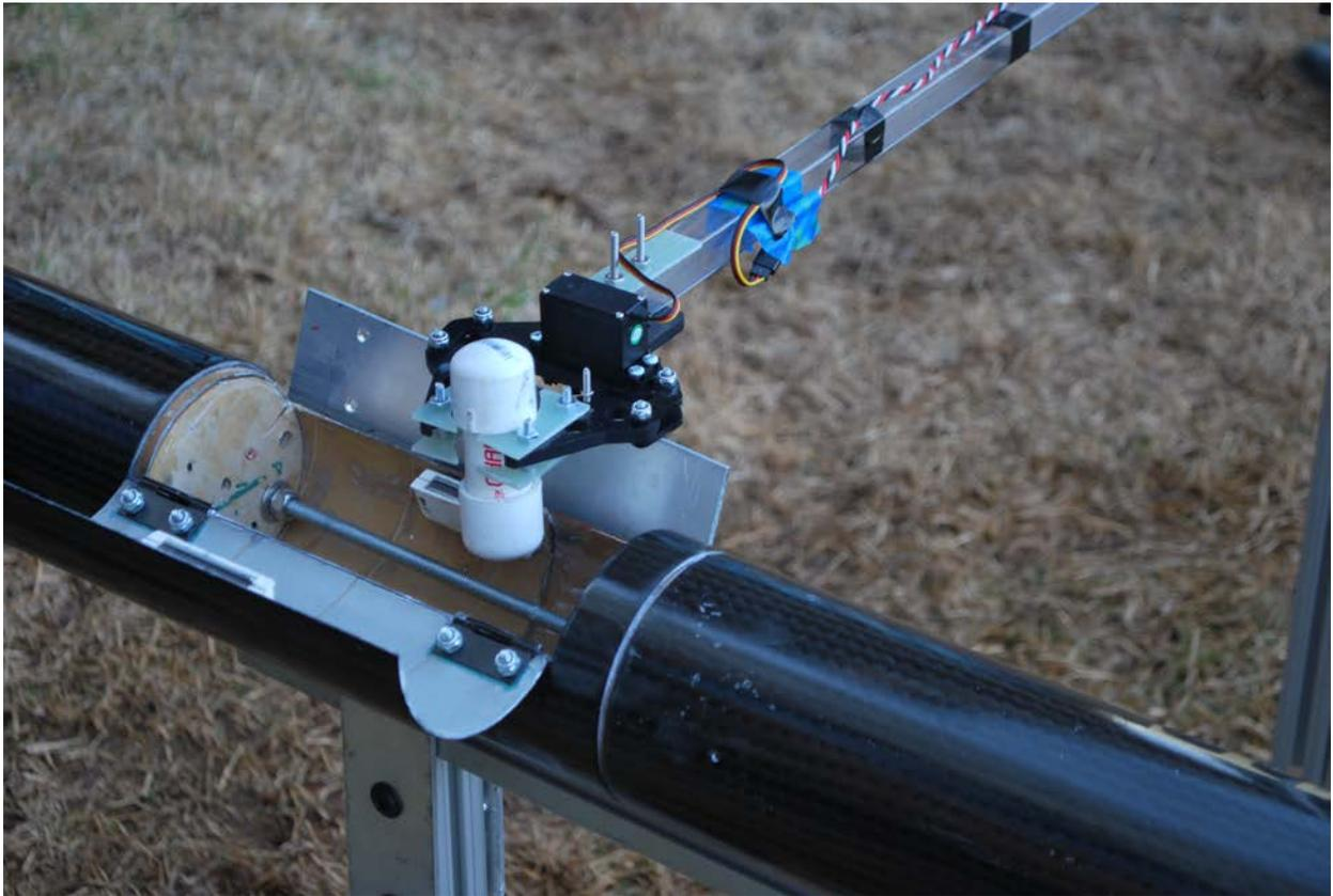
Figure 5: Payload Capture and Containment
